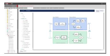
The Sentinet graphical Pipeline Designer and the virtual service processing settings provide User Interface to control the configuration of required message transformations, behaviors and
