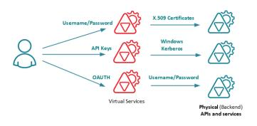
**Security Mediation** (Authentication Schemes mediation). Sentinet supports pass-through and mediated security models when different authentication schemes are implemented for the virtual services and the physical (backend) services. Sentinet supports all industry
